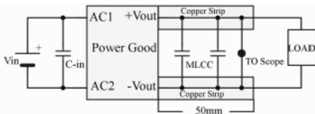
**Figure 1. Measuring Output Ripple/Noise (20MHz bandwidth)**
