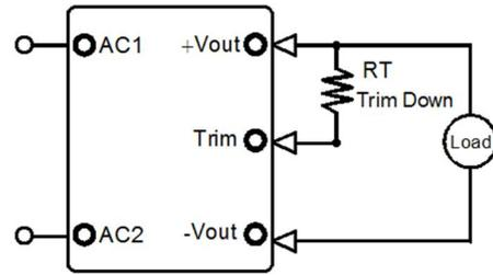
Figure 4. Trim Connections To Output Voltages adjustment For Brick Series
