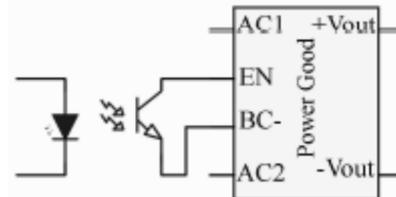
**Figure 2. Driving the Enable Control pin**
