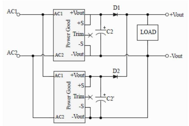
Figure 9. Redundant Connect
