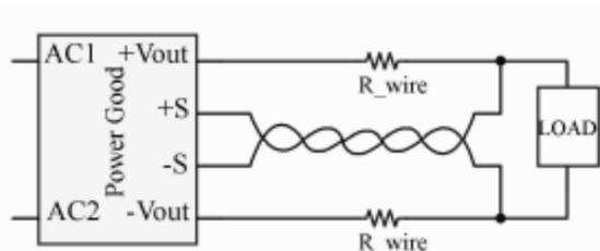
$$[V_{out(+)} - V_{out(-)}] - [Sense(+)] - Sense(-)] \leq 5\% V_{out}$$
